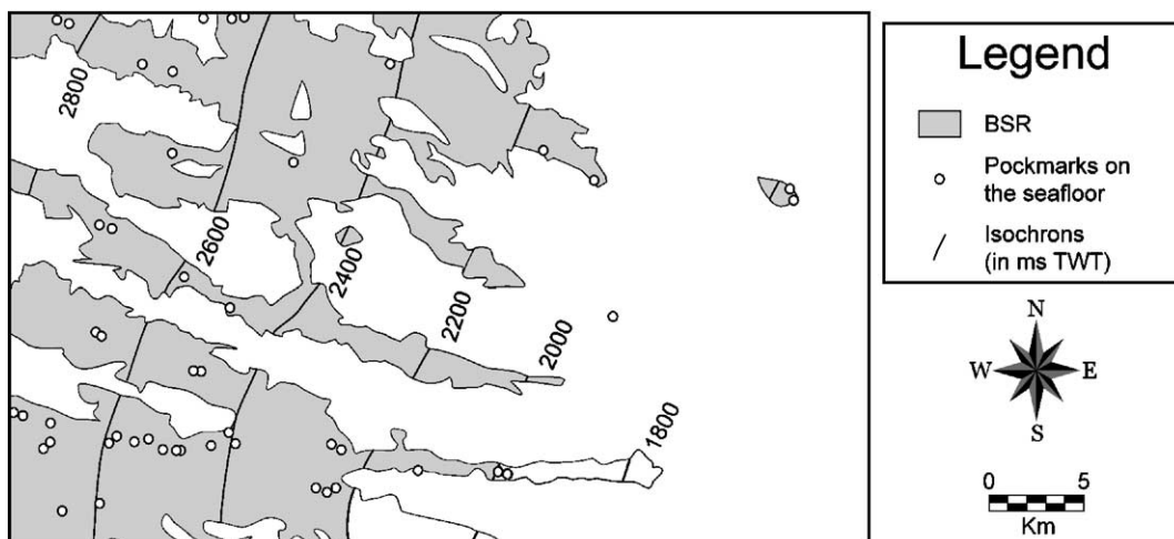
Fig. 10. Isochronal map of a bottom simulating reflector (BSR) visible on 3D seismic sections in the study area. The BSR is dipping towards the WNW and parallels the seafloor slope. Present-day seafloor pockmarks (white circles) with their underlying chimneys are located above the BSR and above areas of high stacking levels of turbidite palaeochannels. This indicates that the fluid pathways are directly linked to the organization of sedimentary bodies (i.e., palaeochannels) and/or to the structuration of the basin.
