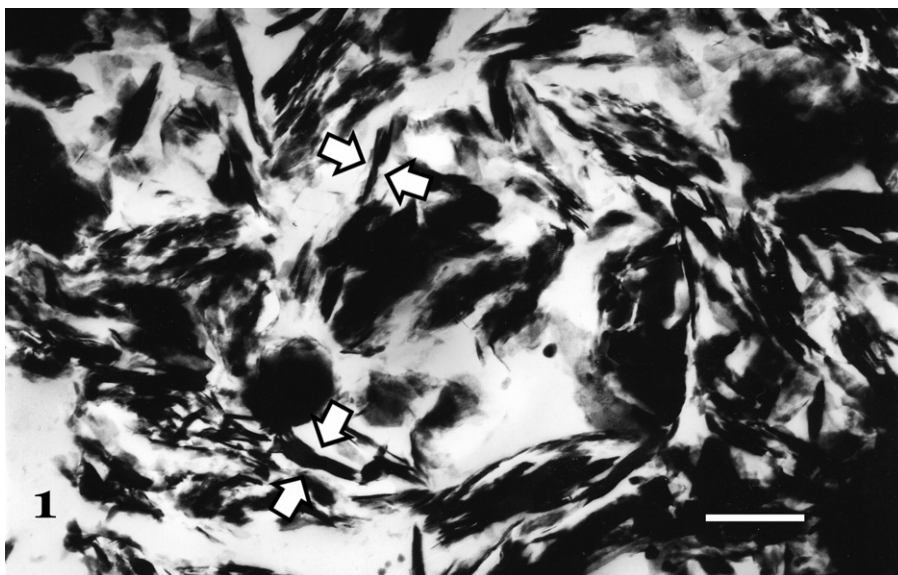
Fig. 1. Illite (90%) and smectite (10%) with 10% chitin. Note the swirled arrangement of clay domains (two representative domains are marked by opposing pairs of arrows). Scale bar = 500 nm.
