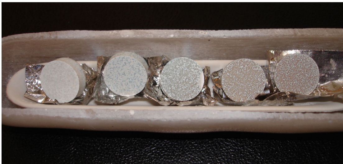
FIGURE 2.7: Heterogeneous pellets of Mn doped fluorapatite (Mn content increases from left to right) after firing on Pt-foil in the feldspar boat inside a cut silica tube.
