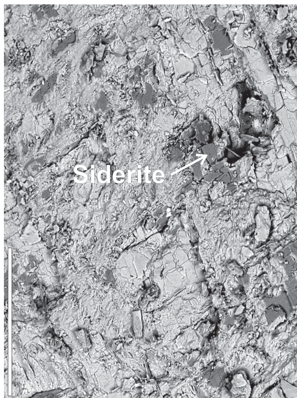
FIGURE 4. SEM image of siderite after partial decarbonation. Patchy areas of siderite remain in an otherwise massive matrix of magnetite. The morphology of the siderite is preserved in the magnetite. (White scale bar = 200 μm).
