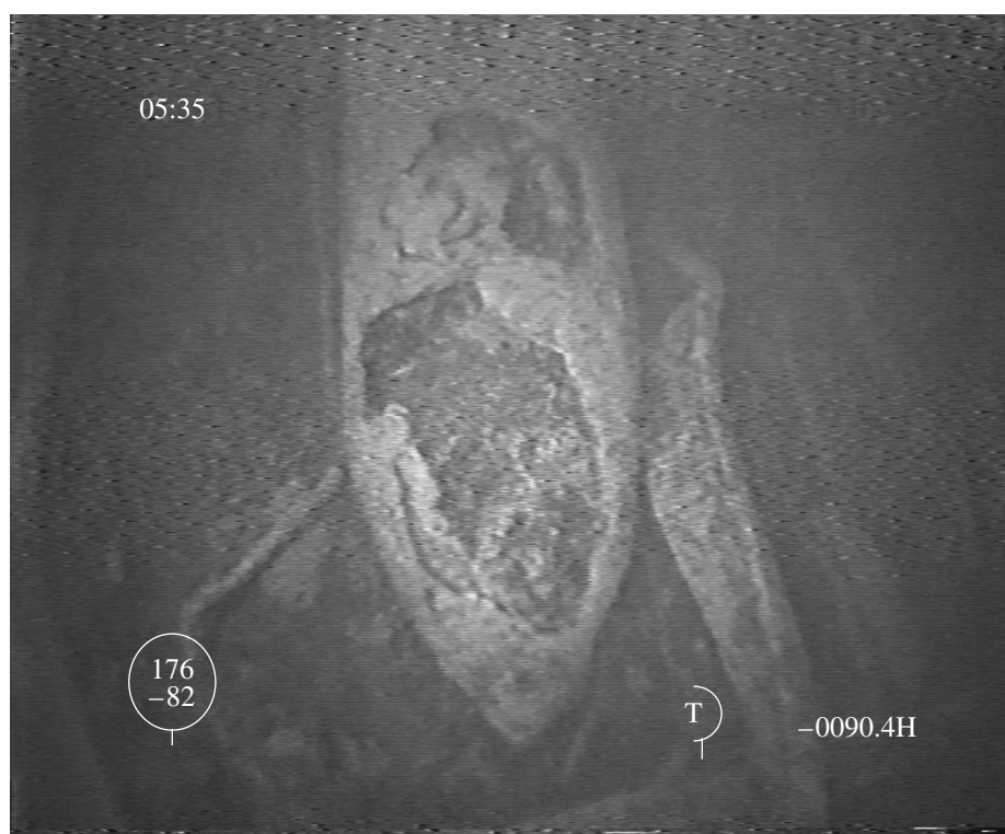
Fig. 9. Corroded steel shell of an aircraft bomb that rested for 55 years on the floor of the Bornholm Deep, Baltic Sea, billed with warfare poisonous agents [1].
