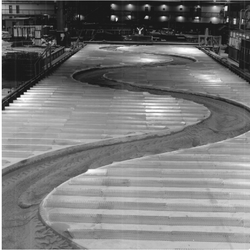
Fig. 10. Example of an experimental compound channel in the Flood Channel Facility (FCF). Roughening elements are shown on the floodplain. The flume tank shown is 60 m long and 10 m wide, of which the experimental channel occupies a length of 35 m. At high flow, overbank fluid flows strongly parallel to the sides of the flume, whilst within-channel flow moves in a sinuous path through the main channel. From Wormleaton et al. (2005). Reproduced with permission from ASCE.
