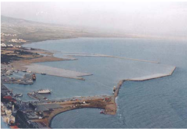
Photo 14 Aerial view of the port of Alexandroupolis City with its new extension eastwards in 2004–05. The SW directed sea waves and eastern deposition coast, up to Evros River Delta, is shown as well
