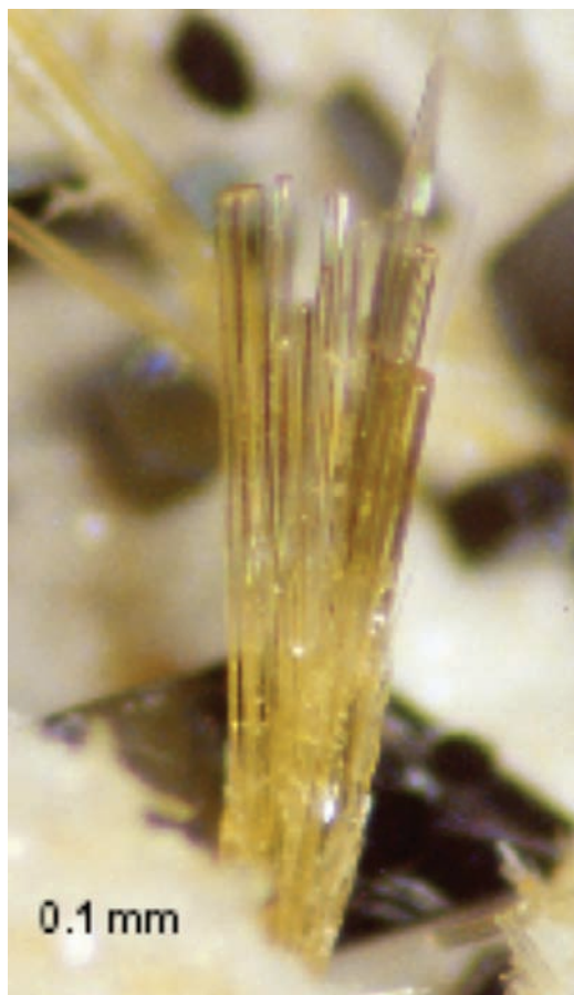
FIG. 1. Optical micrograph of fluoro-edenite studied by \mu -Raman and \mu -FTIR spectroscopy.
