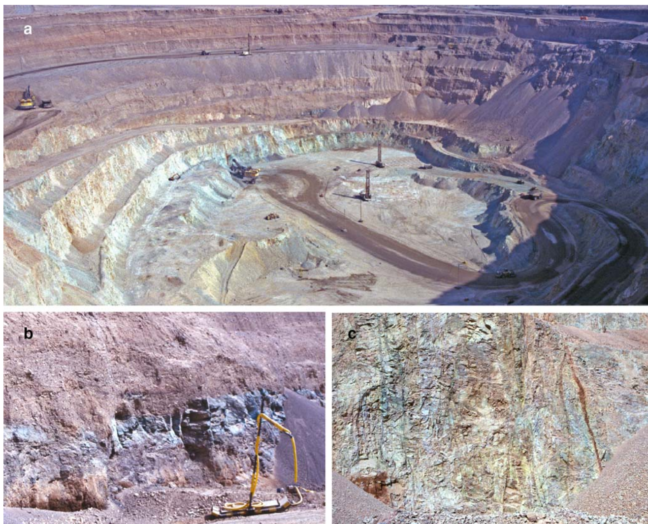
Fig. 9 a General view of Radomiro Tomic pit, February 1999. Green colour is atacamite. There is considerable relief on the top of the oxide zone, being highest to the right of the slumped gravels. b Chrysocolla mineralization extending into gravels from zone of atacamite depletion to the right. Water of meteoric origin dripping from the pit wall was
