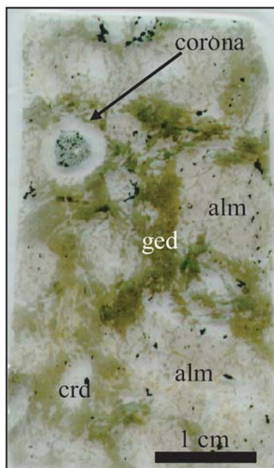
FIG. 3. Scanned image of a thin section showing a corona structure in gedrite – cordierite – garnet gneiss composed of a core of aluminous minerals (hercynite, staurolite, corundum, sillimanite, cordierite, and h ogbomite) plus ilmenite separated from gedrite and almandine by a moat of cordierite.
