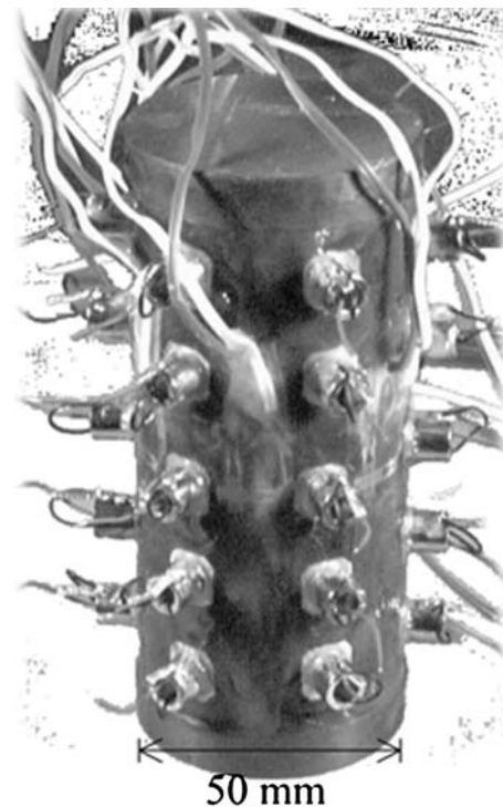
Fig. 2 Photograph of rock sample with mounted PZT sensors
