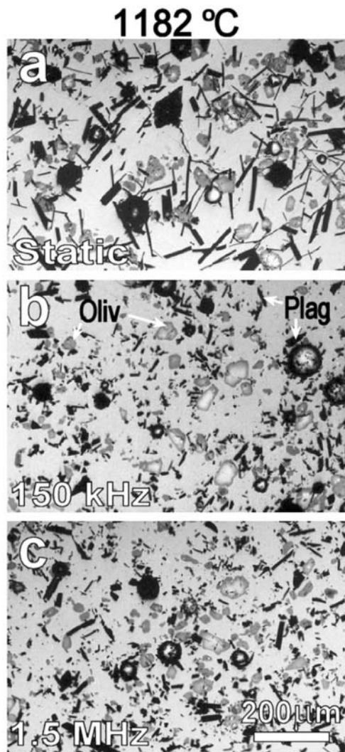
FIGURE 4. BSE images of (a) static experiment Ex1s, (b) 150 kHz experiment Ex5v, and (c) 1.5 MHz experiment Ex2v. Black and/or white circles are vesicles, black lath shapes are plagioclase, medium-gray crystals are olivine, and the light-gray background is glass. All experiments were conducted at 1182 °C. Scale bar is 200 micrometers and all photos are at the same scale.
