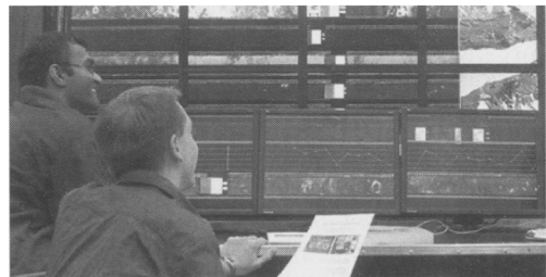
Fig. 8. The Corewall core data visualization system. Corewall uses high-resolution tiled LCD displays to show images of core sections along with discrete data streams of measured parameters downcore and nested images, allowing rapid multi-disciplinary interpretation. Corewall users can also link and download data from remote databases, allowing access to dispersed datasets for interpretation. Sophisticated data visualization tools like Corewall will lead to the development of amplified collaboration environments for core analysis. (Reproduced courtesy of Arun Roa and the Corewall Consortium).
