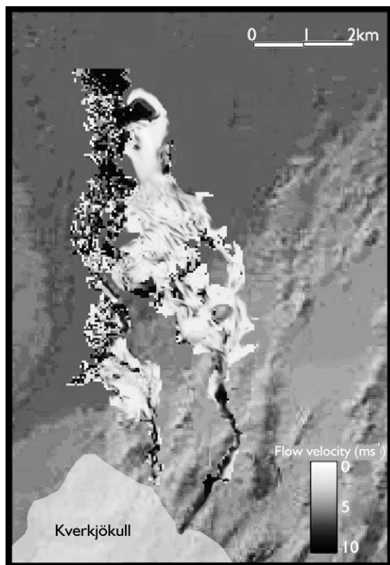
Fig. 3. Example of flow initiated in two channels simultaneously, in the same area as depicted in Fig. 2. Variation in flow velocity demonstrates higher velocities in narrow and steep upper reaches, accelerated velocities over spillways, and braided sheet flow on unconfined outwash area
