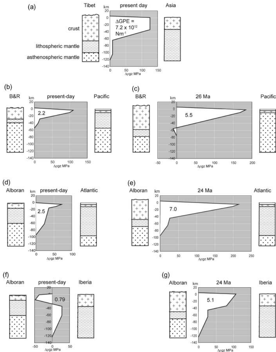
Fig. 5. Plots of gravitational potential energy difference ( \Delta GPE ) between hinterlands and their surroundings. Each plot shows the difference in lithostatic pressure ( \Delta pgz ) in MPa (horizontal axis) with depth in km (vertical axis) between a hinterland area and its immediate surroundings. The integral of \Delta pgz with depth (area under the curve, in white) is the \Delta GPE : values are shown in units of 10^{12} \text{ N m}^{-1} . It should be noted that some curves show negative contributions (left of zero line) as well as positive. (a) India v. Asia at present day; (b) Basin and Range (B&R) v. Pacific ocean lithosphere at present day; (c) Basin and Range (B&R) v. mid-ocean ridge at time of ridge–trench collision at 26 Ma; (d) Alboran v. Atlantic at present day; (e) Alboran v. Atlantic at start of extension at 24 Ma; (f) Alboran v. Iberia at present day; (g) Alboran v. Iberia at 24 Ma.
