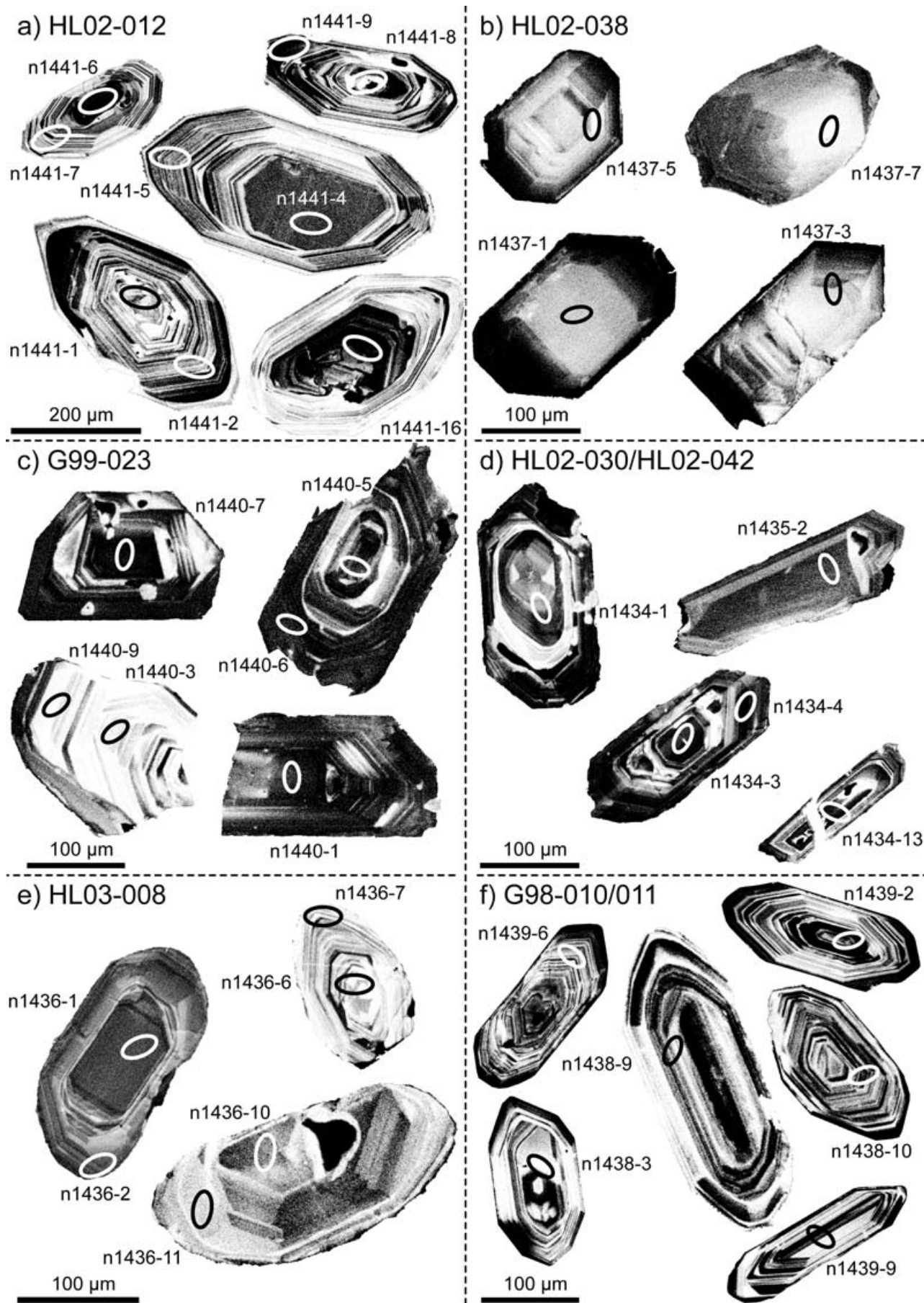
Figure 10. (a–f) Cathodoluminescence images of zircons. Analysed spots are marked by an ellipse.
