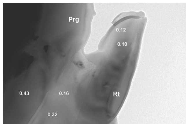
Fig. 10. Ti content (apfu) in the analyses of the brown amphibole host, obtained at variable distance of the rutile (Rt) inclusion.
