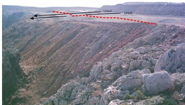
Fig. 12 A photo of the Kouroupitos' gorge showing the limit between the ground (limestone) and the deposited wastes. ERT lines 4 and 5 together with the boundary between paleorelief and current slope ( dotted line ) are also depicted
