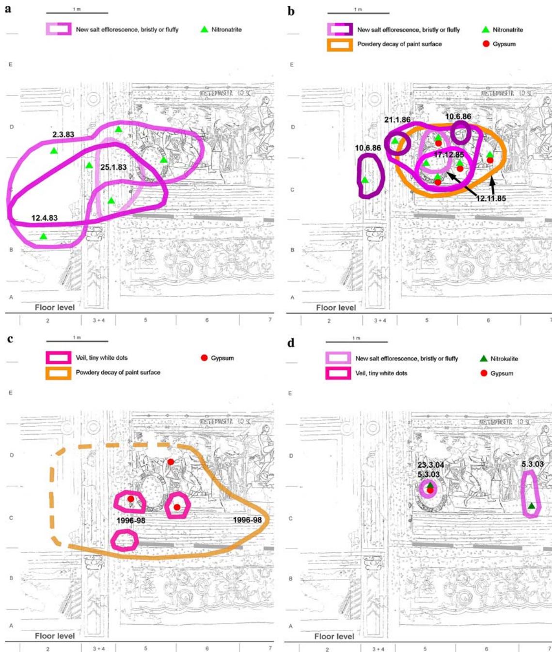
Fig. 4 Damage evolution on a section of the north apse in the convent church of Müstair, exemplified by four stages from 1983 to 2004. a Illustrates a seasonal cycle of nitronatrite efflorescence during the heating period of 1982/83. It started in the centre of an area that was affected by this salt earlier (Fig. 3), then it spread and retreated with irregular outlines. b In 1986, gypsum efflorescence developed associated with powdery decay of the paint surface. At the same time, nitronatrite efflorescence was
