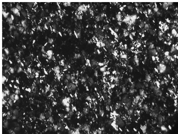
Fig. 5. Cross-polar photomicrographic view of fossil-bearing siltstone. Two populations of grains are present, larger (and darker) quartz grains and smaller, elongate, and lighter-appearing elongate grains. Width of view 400 \mu\text{m} .
