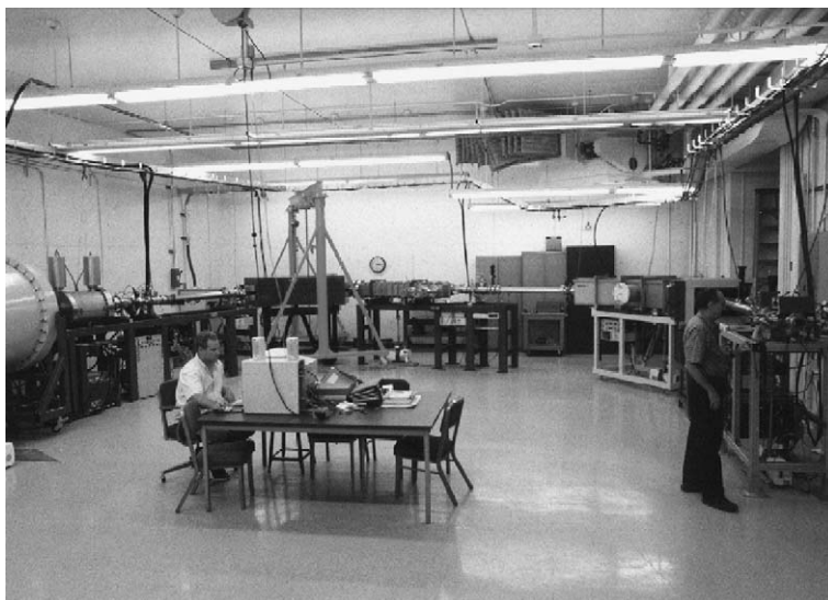
Fig. 3. Photograph of the high-energy beam line and detector system of the University of Arizona 3 MV Pelletron accelerator mass spectrometer.
