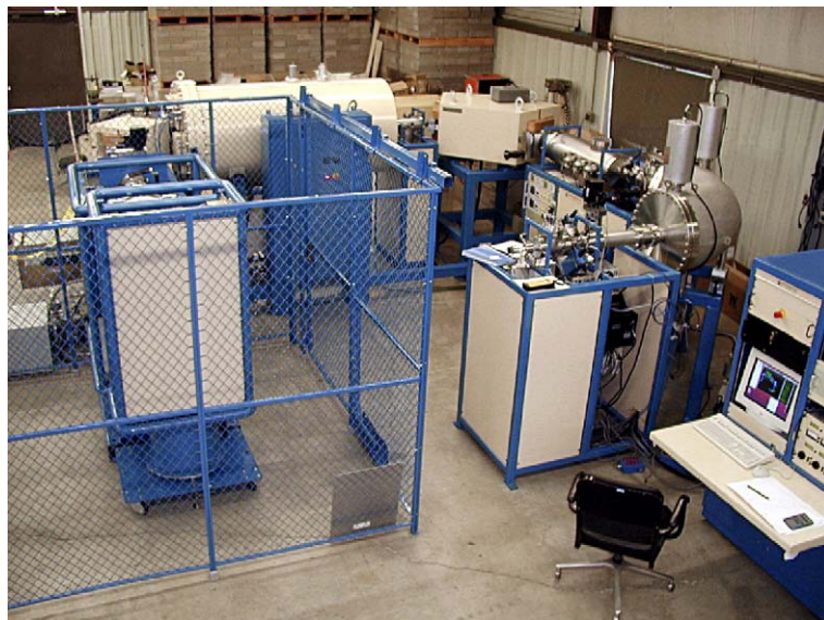
Fig. 5. Photograph of the 0.25 MV single-stage accelerator mass spectrometer, developed for the University of Lund. Courtesy of National Electrostatics Corporation.
