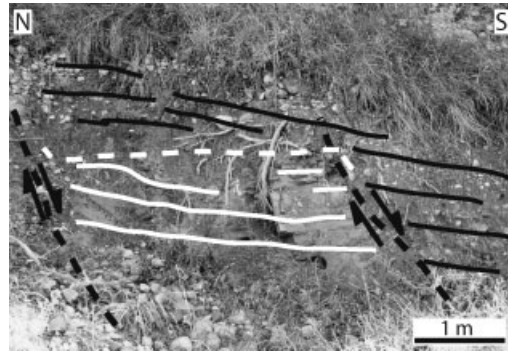
Figure 5. Syn-sedimentary faulted contact between the lower conglomerates (black solid lines) and the Eocene substratum (white solid lines). Faults (black dashed lines) dip 220/84 and 225/64 (azimuth/dip). White dashed line marks Messinian erosional surface.
