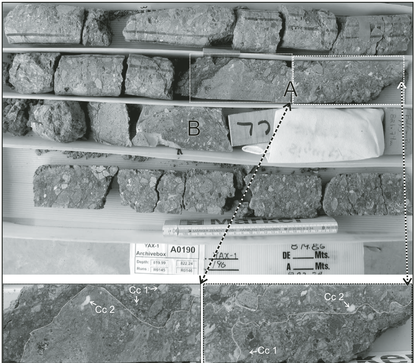
Figure 6. Photographs of the basal Lower Sorted Suevite drill core box that contains core pieces from 819.99 m to 822.24 m. Two melt breccia intercalations occur at 820.9 m (A) and 821.4 m (B). Cc 1 indicates micritic limestone clasts and Cc 2 indicates recrystallized limestone clasts in core pieces from (A).
