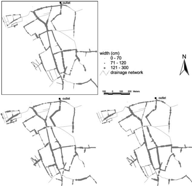
Figure 10. Width data on top-left depicted by dark grey points with legend on top-right. The 2 sub-figures down are examples of simulated values depicted with the same legend as for the actual ones.
