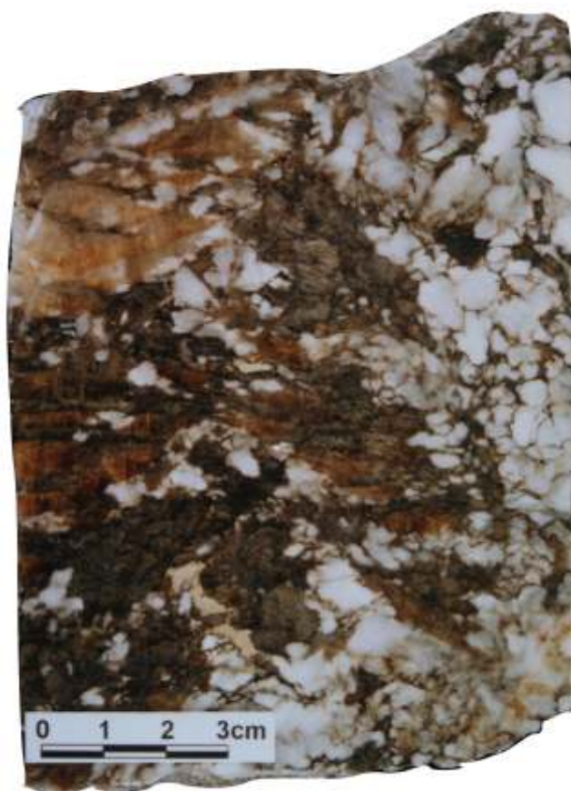
Fig. 3. Selenitic gypsum partly replaced by nodular anhydrite
