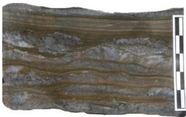
Fig. 4. Organic-rich claystone with anhydrite laminae and lenses composed of pseudomorphs after lenticular gypsum crystals
