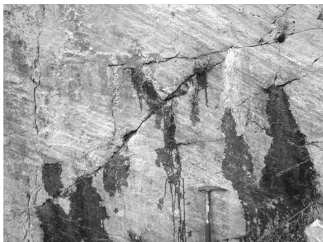
Fig. 1 Fractured gneiss outcrop near Lom, Norway, with water flows from water-conducting fractures. Interconnected fracture network with fracture density of 4 \text{ m}^{-1} . Scale: hammer
