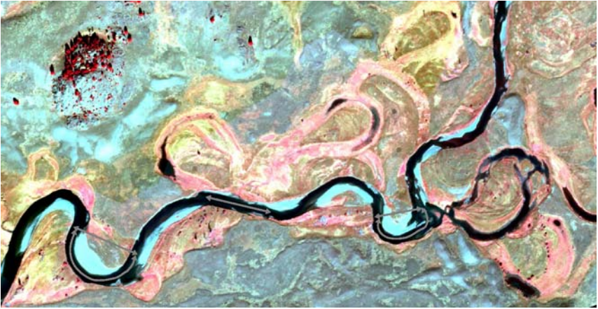
Figure 1. Meandering section of Slough Creek, Yellowstone National Park, USA. In areas of high curvature, Euclidean distances between pairs of points underestimate the along-channel path length, as shown in the bends at the left and right. In relatively straight channel segments (center), the discrepancy between Euclidean and along-channel distances is smaller. Flow is from right to left.
