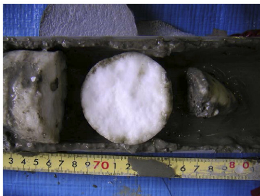
Fig. 5. Photo of massive gas hydrate collected from PC11 at \sim 1.7 mbsf. Analytical results of melt waters from such gas hydrate samples are indicated as “GH” in Table 1.
