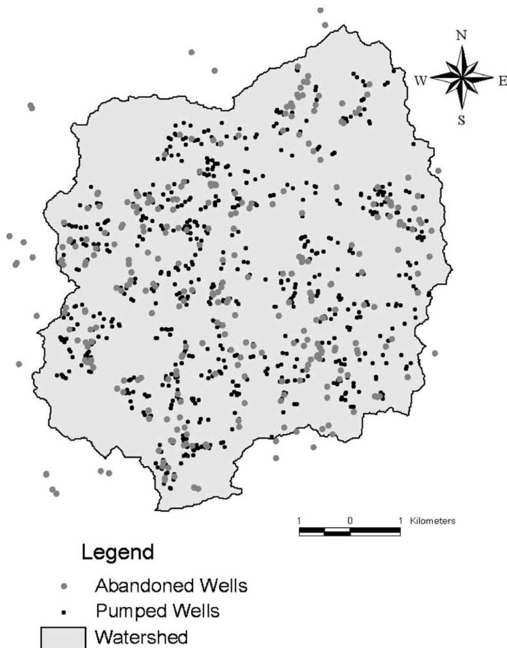
Fig. 3 Study area with location of pumped wells and abandoned wells used as piezometers
