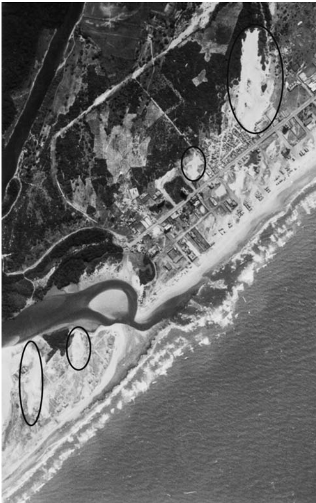
Fig. 17 Dune movements ( ellipses ) toward vegetation, streets, and building areas in the estuary area of the Cocó River
