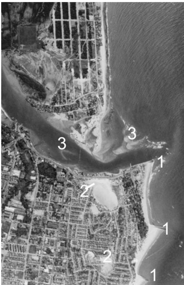
Fig. 6 General view of the estuary of the Ceará River: 1 dikes built (moles) to control erosion/sedimentation processes, 2 dune movements toward the road and residences, and 3 sediment load transported by Ceará River
