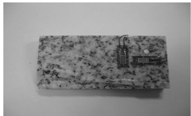
Fig. 2. Photograph of the granite specimen with adhered strain gauge.
