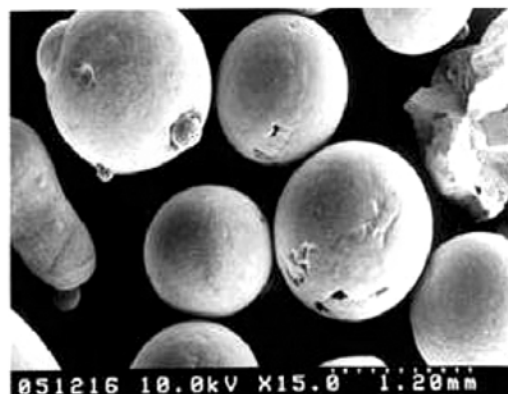
(b) SEM (x 15) picture of atomized slag
