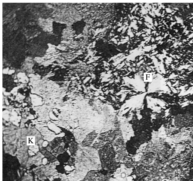
Fig. 5. Replacement of kotoite marble by fluorite laths (F). Baia Roshe deposit, Romania. Sample R-040, transparent thin section. Magnification 25 \times .
