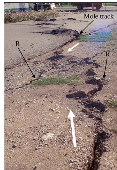
Fig. 5. Ground view of surface faulting at Las Manosas hardware store, where dextral R shears are connected by mounds at restraining stepovers. All these features were nicely developed and well preserved in paved lateral yard. For location, refer to Fig. 3.
