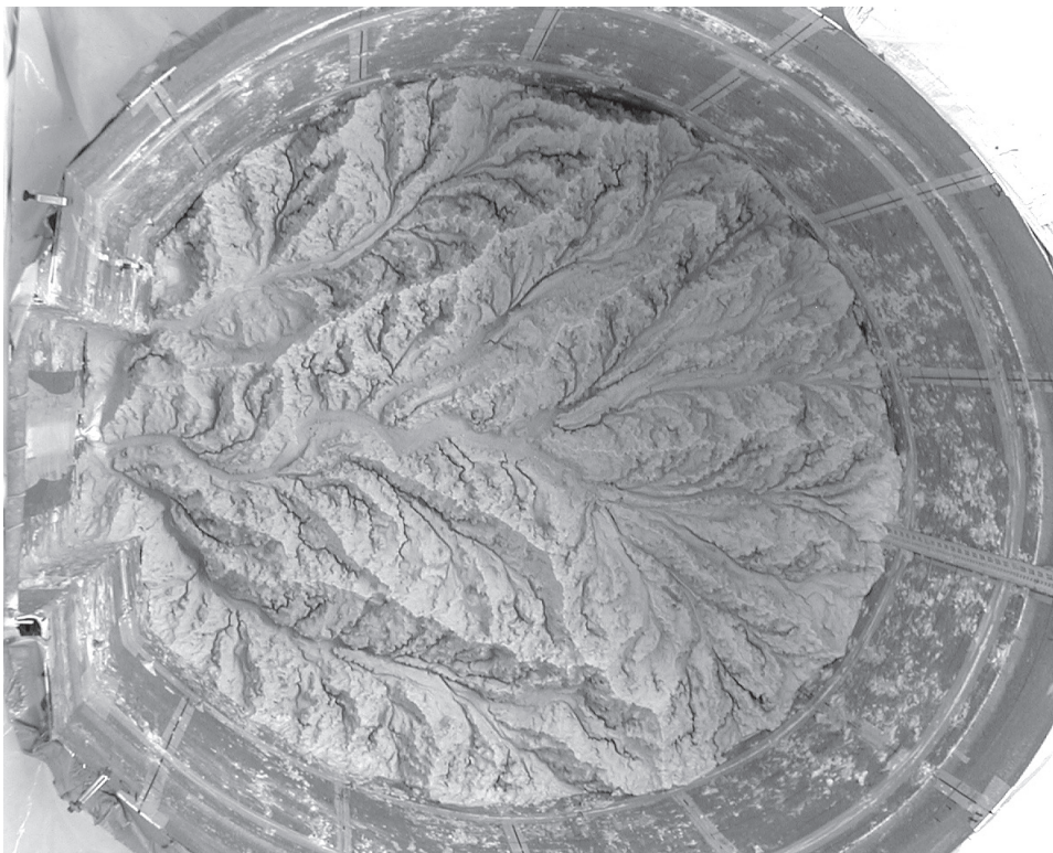
Figure 3. Vertical view of the dendritic pattern of the drainage network. The photo was taken long after complete dissection of the initial surface (note rind near the top of the basin walls) at run time 62:13 h. Outlet is at left center. Basin length (left to right) is 98 cm; basin width (top to bottom) is 86 cm.
