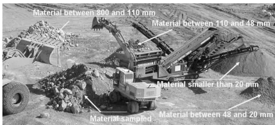
Fig. 5. General view of the mobile screen, front loader, excavator and piles
