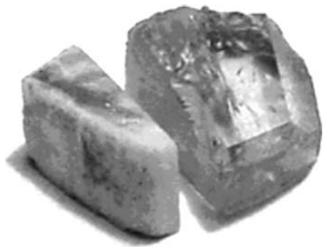
Fig. 15 Two pieces of topaz K4, natural ( right ) and annealed during 1 h at 1,050°C ( left ). A part of the annealed sample transformed to non-transparent milky-white material. A distinct zone of the newly formed material is obviously related to one of the {001} prism face
