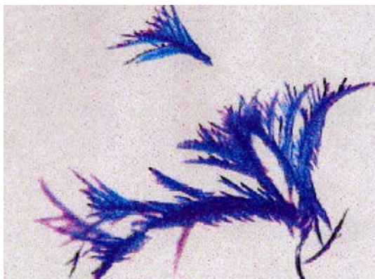
Fig. 7 Microphotograph of blue dendritic \text{CoHg(SCN)}_4 crystals (250 \times )
