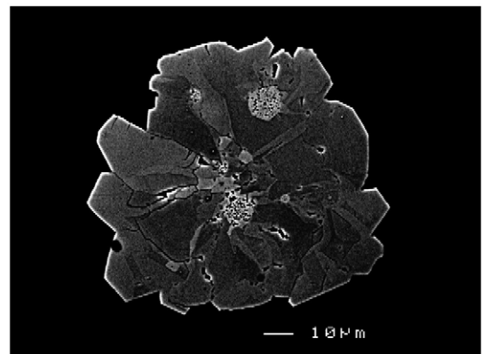
Fig. 6. Backscattered electron microscope image of a euhedral pyrite crystal. Two framboids can be seen (at center and at top) within the crystal. Note 10 micro-meter scale bar.
