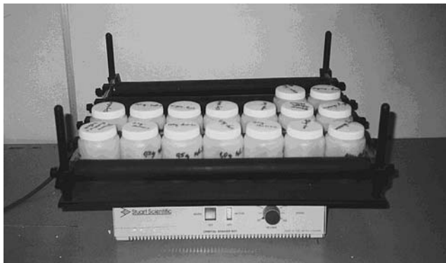
Fig. 9 Orbital shaker used in the batch equilibrium tests
