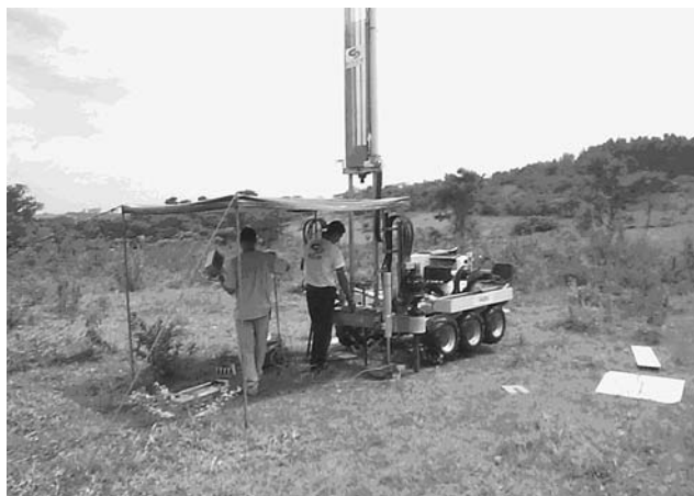
Fig. 5 Self-anchoring, multi-purpose push platform carrying out piezocone tests at Bauru’s MSW disposal site
